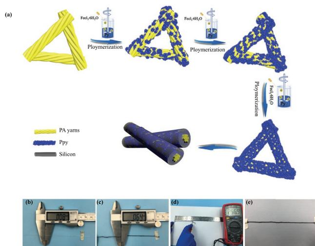
**Figure 1.** Schematic diagram. a) Schematic showing the preparation of PA-PPy yarn and EMS-TENG. b,c) The diameter of PA and PA-PPy<sub>7</sub> yarn. d,e) Resistance of PA-PPy<sub>7</sub> yarn and the photograph of EMS-TENG.
